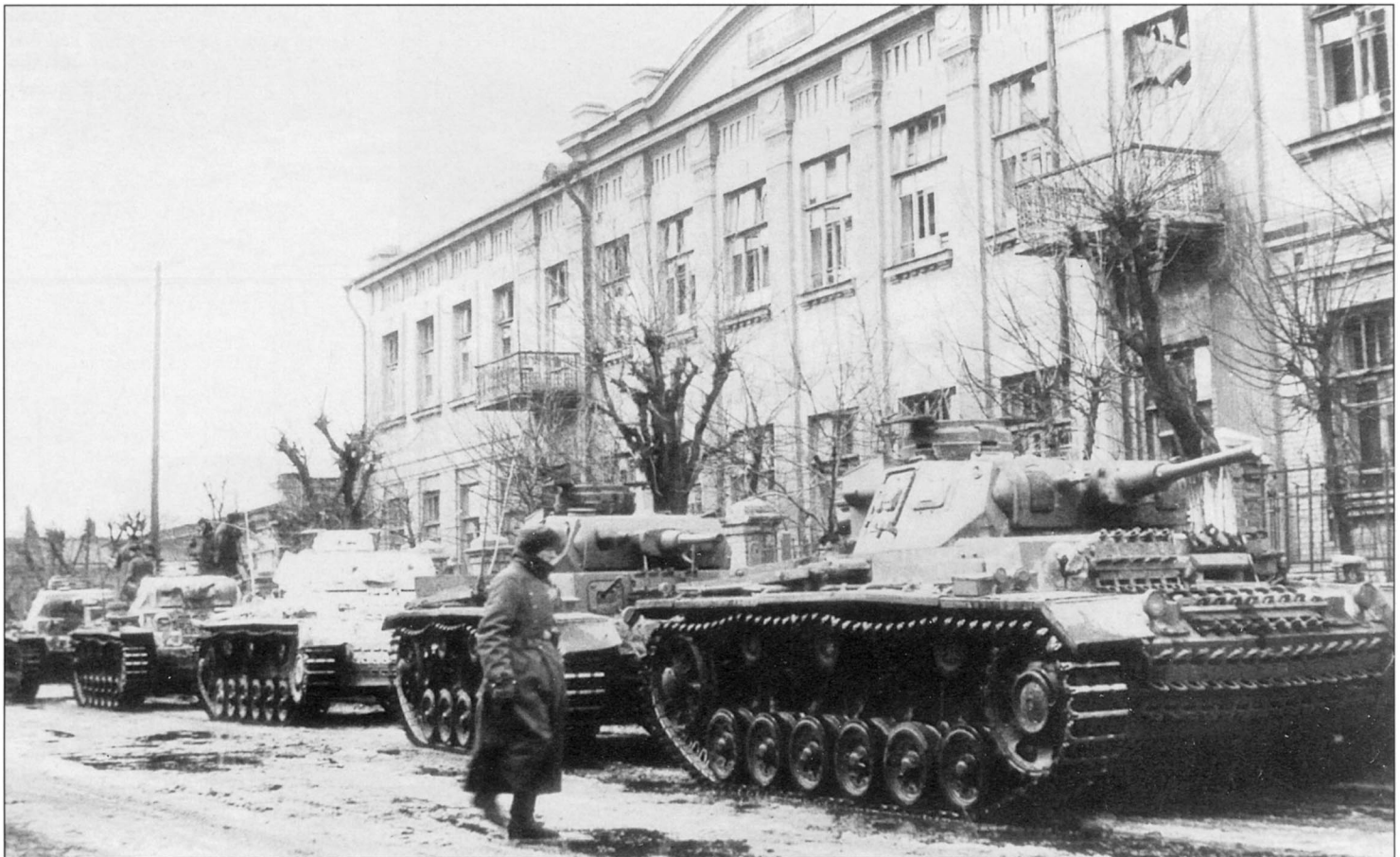
A number of Pz.Kpfw. IIIs of different production lots gather in a Soviet town. The third vehicle appears to be brand-new since the camouflage on all the others has worn off. Though upgunned with the L/42 gun prior to "Barbarossa", these tanks became obsolete on the battlefields of 1942.
