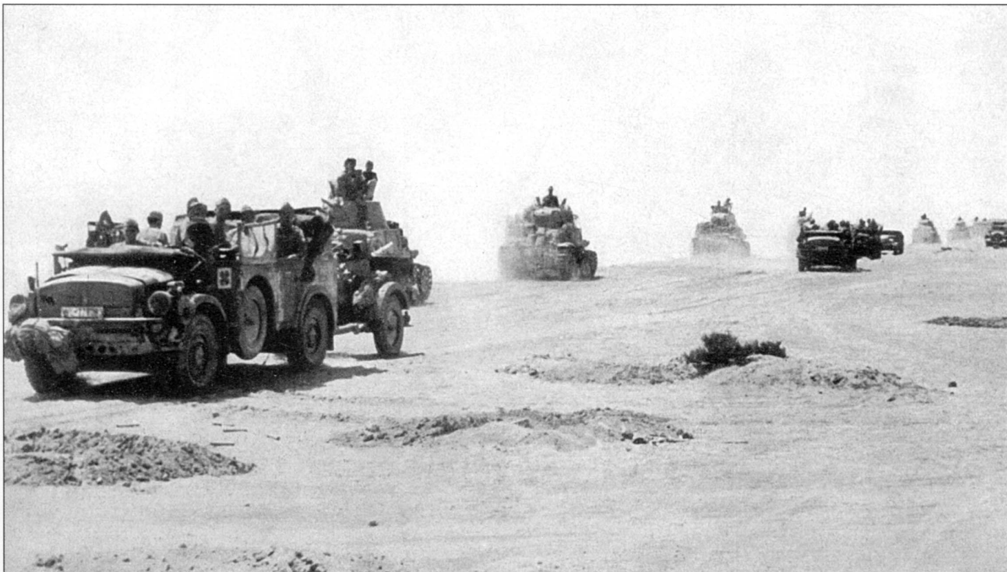
A German anti-aircraft platoon, which is equipped with 2cm Flak 38 guns, passes a column of Italian tanks in the barren North African desert. The M13/40 tanks were no match for their British adversaries. The Kfz. 69 (Horch) is equipped with anti-flare covers over the windscreen.
