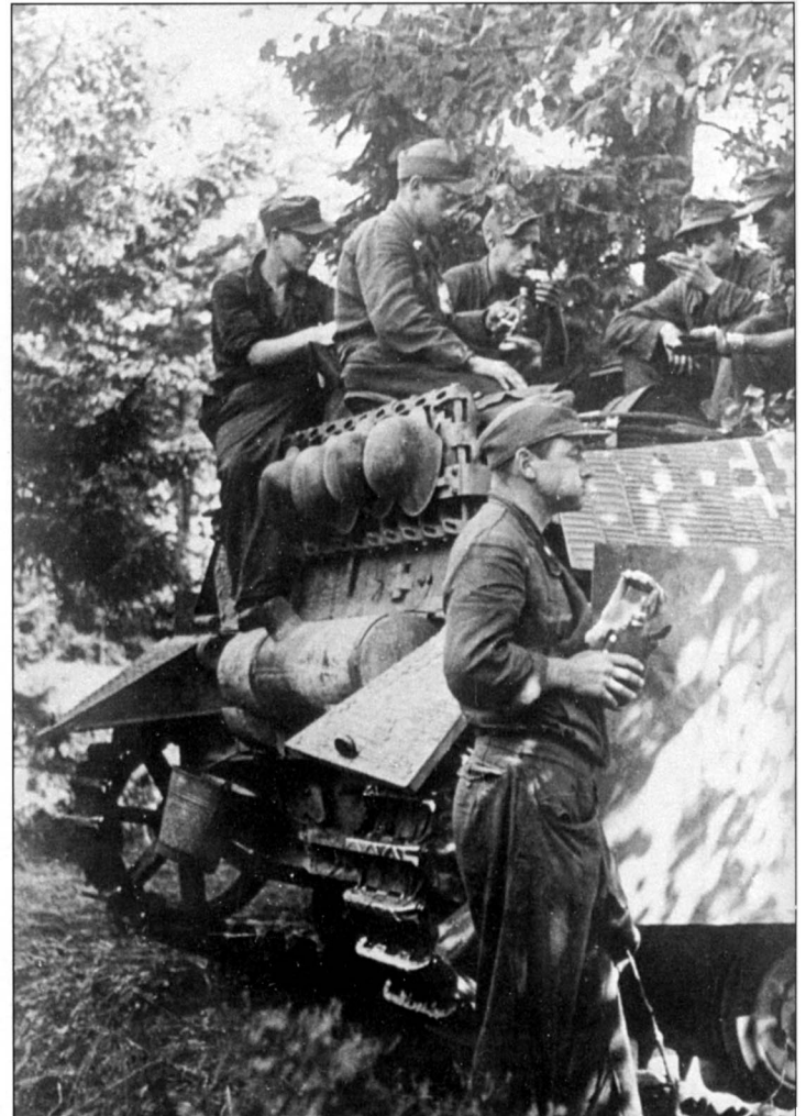
The crew of this Jagdpanzer IV (7.5cm L/48) of Panzerlehrdivision enjoys a meal on top of their vehicle. The spare track links fitted to the rear indicate that this is a late production tank hunter. Zimmerit is once again visible on all armor plates.
