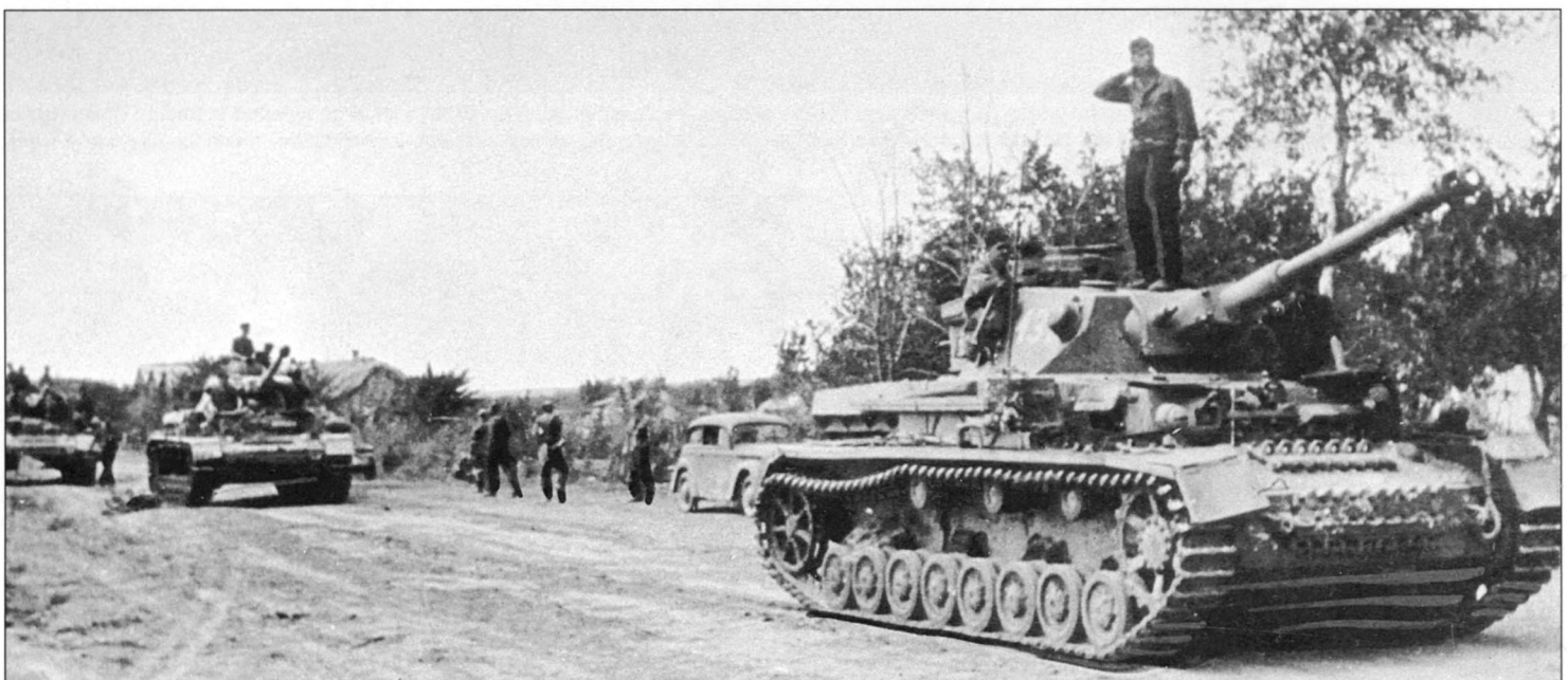
In the late spring of 1942, the first Pz.Kpfw. IVs fitted with the high velocity gun seen here were delivered to the front-line units. This Ausf. G was able to deal with all Soviet and English tanks at distances up to 700 m (765 yards). The tank at right is finished in plain dark gray, with the turret number '431' being painted in white.
