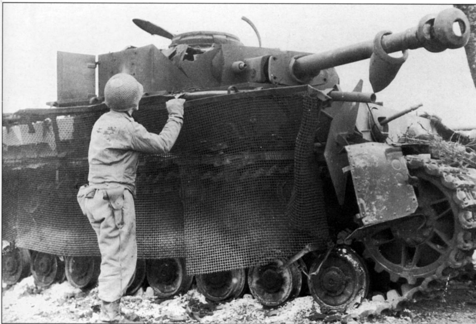
A fine view of a late-production Pz.Kpfw. Ausf. J. The tank was hit at the turret edge, but probably some other rounds penetrated its armor and caused a fire. All rubber coatings have burned down to ash. The G.I. is holding on to a wire mesh screen known as a Thoma Schild (Thoma shield), which was an antibazooka shield.
