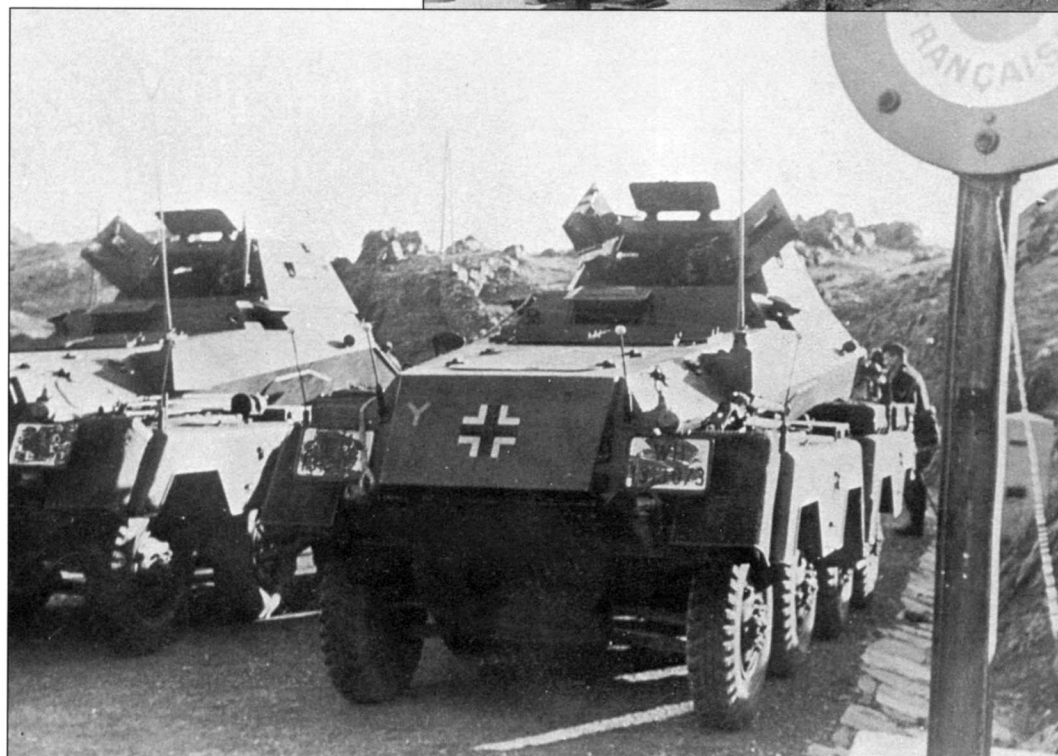
Many armored units were sent to France for refitting. These armored cars of 7.Panzer-Division are late production Sd.Kfz. 232s sporting the 1.3m star antenna instead of the prominent frame antennas. The vehicles are still finished in plain dark gray.
