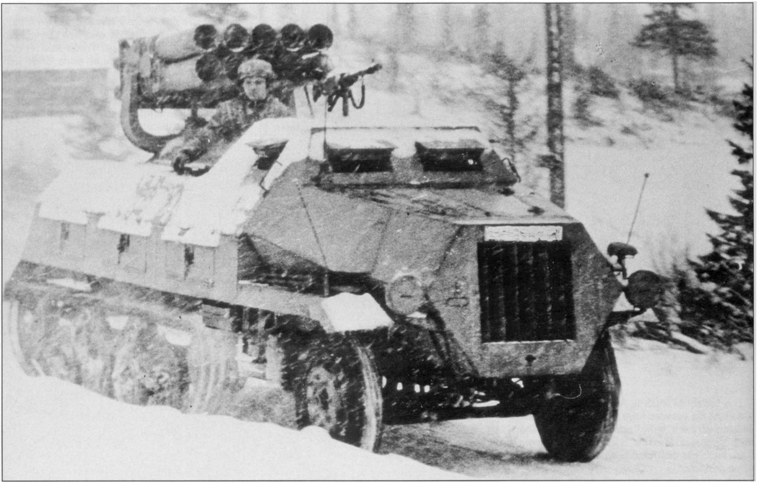
A valuable support weapon, this 15cm Nebelwerfer rocket launcher mounted on a 2-ton Maultier moves steadily through the snow. Fully armored, this vehicle was very successful. The vehicle commander stands in his open hatch. Note the MG34 mounted for close combat defense.
