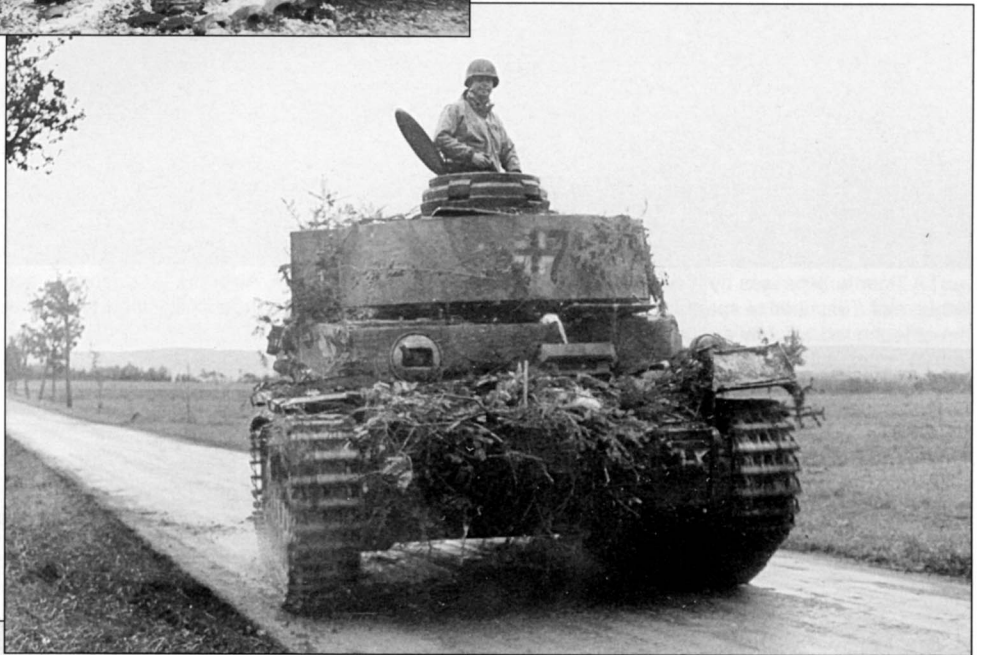
This Pz.Kpfw. IV, which was captured intact by US troops, is being moved back to the rear for evaluation. Although obsolete, the Pz.Kpfw. IV, with its 7.5cm L/48 gun, was able to knock out any Allied tank at normal combat ranges.
