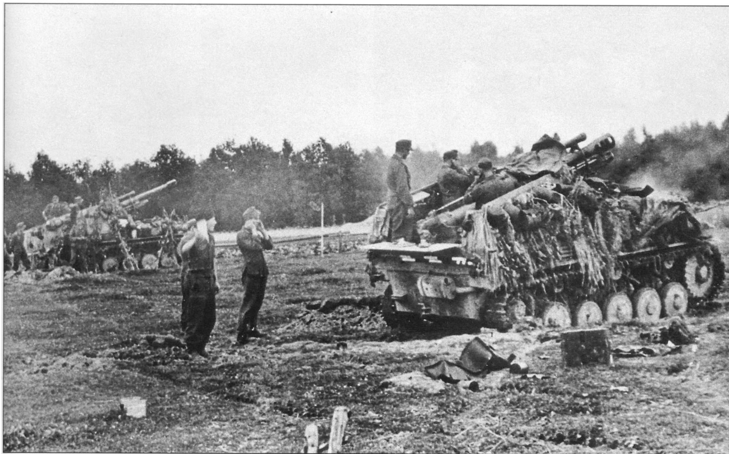
Introduced in 1943, the Wespe (wasp) self-propelled gun significantly improved the mobility and effectiveness of German field artillery. The gun in the foreground has just fired a round, and its 10.5cm barrel is seen at full recoil. Note that all personal belongings of the crew are stowed outside; the cramped interior did not leave any space for non-essential items.
