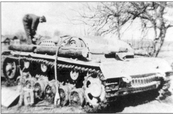
This battle-proven StuG III Ausf. D carries a lot of extra equipment. This practice was necessary because the assault guns were so cramped inside. Two wooden beams were stowed on the fenders for recovery purposes. Spare tracks, additional running wheels and Soviet towing ropes complete the load of equipment.
