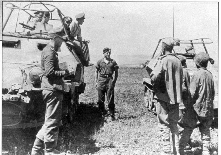
Officers of a Panzergrenadier unit interrogate Russian prisoners of war. The vehicle at left is a Sd.Kfz. 251/6 (Ausf. C), the one at right a Sd.Kfz. 250/3. Both vehicles were prime targets for enemy guns because they were easily recognizable from a distance as command vehicles due to their conspicuous frame antennas.
