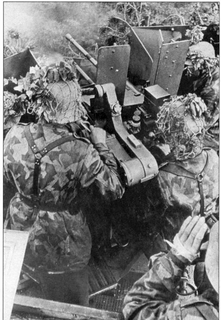
Engaging a ground target, this quadruple Flakvierling fires with all barrels. Offering a high rate of fire, these guns were very effective against soft targets. The loading of ammunition was complicated, however. Each gunner had to take care of two guns, changing the 20-round magazines every few minutes. This procedure was not easy as both gunners had to coordinate the exchange with the gunner.
