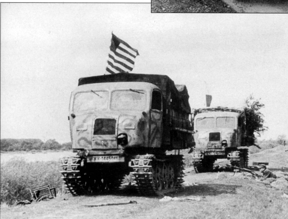
These two Raupenschlepper Ost (RSO) tracked vehicles were pressed into service by US troops. Intended for the rough conditions of the Eastern Front, it was a slow mover with a maximum speed of 15-20 km/h (9-12 mph). However, its cross-country mobility was legendary. A large American flag is displayed to protect the Americans on board from a fatal case of mistaken identity.
