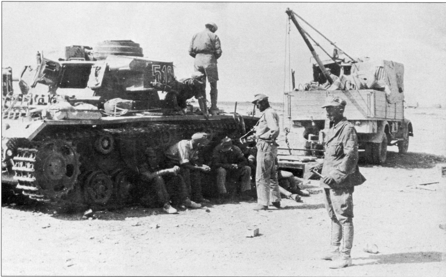
In this photo a 3-ton truck, which has been converted to a workshop, is employed to remove the engine cover of a damaged Pz.Kpfw. III Ausf. J. Apparently, the engine broke down, which was quite a frequent problem in the heat of North Africa. Note how the tank crew members escape the sun by sitting in the shade created by their vehicle.
